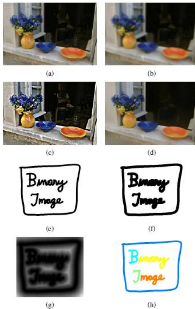
Figure 3.11 Some neighborhood operations: (a) original image; (b) blurred; (c) sharpened; (d) smoothed with edge-preserving filter; (e) binary image; (f) dilated; (g) distance transform; (h) connected components. For the dilation and connected components, black (ink) pixels are assumed to be active, i.e., to have a value of 1 in Equations (3.44–3.48).
