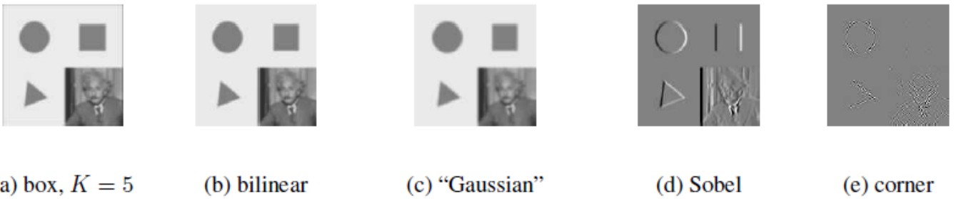
Figure 3.14 Separable linear filters: For each image (a)–(e), we show the 2D filter kernel (top), the corresponding horizontal 1D kernel (middle), and the filtered image (bottom). The filtered Sobel and corner images are signed, scaled up by 2\times and 4\times , respectively, and added to a gray offset before display.
