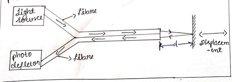
working => sight forom the source passes through one optical fibre and incident on the target. The neflected light neaches the photodetector through another optical fébre. Light reflected from target and collected by the detection is a function of the clisplacement of the target may be negestered at the optical detector
