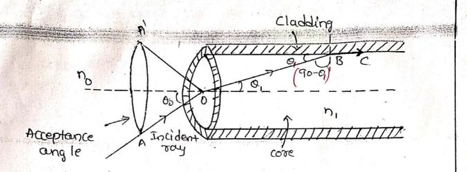
When a ray of light 'AO' is incident at 'O' at an angle 'O'. This ray undergoes refraction at an angle 'O'. In the core and further proceeds to fall at critical angle of incidence [≈(90-0,)] at 'B' . On the interface blue core and cladding. The ray 'OB' grazes along 'BC'
