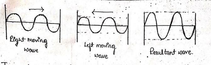
To get constructive interjerence, the distance between the merror should be (L) an integral multiple of 2/2.
